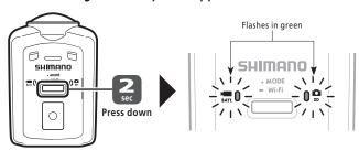
• Turn on the camera and hold down the MODE button until you hear a beep, then the LED turns green to indicate that the camera is transmitting Wi-Fi signals.
