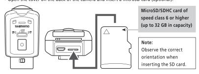
• If you try to operate the camera without an SD card mounted, a series of warning beeps sound to indicate that an SD card is missing. The camera cannot be used without an SD
